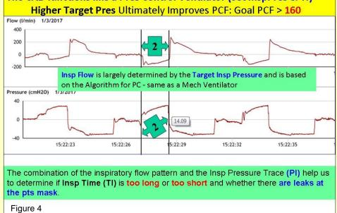
target pressure and more patient demand both result in increased flow and resultant tidal volume. The device also has three flow settings (low, mid, high) that act to control how rapidly the flow valve opens –a function identical to the pressure slope setting on a mechanical ventilator.
