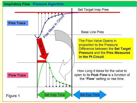
the same algorithm or logic to control the flow during inspiration. The valve (in this case the **blower motor in the CAD**) is controlled by a logic sequence or "algorithm" that determines the amount of flow into the lung: 1a) A target inspiratory pressure is
